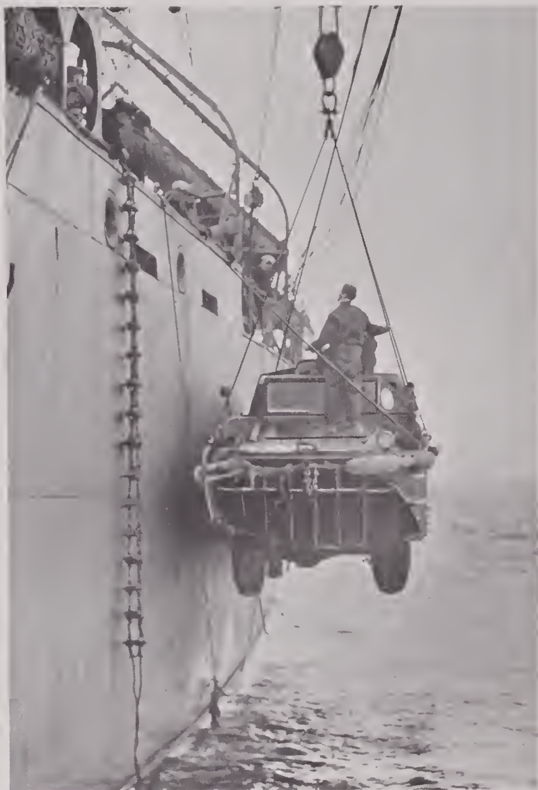
FIGURE 104. Liberty ship jumbo boom lifting DUKW from water.
